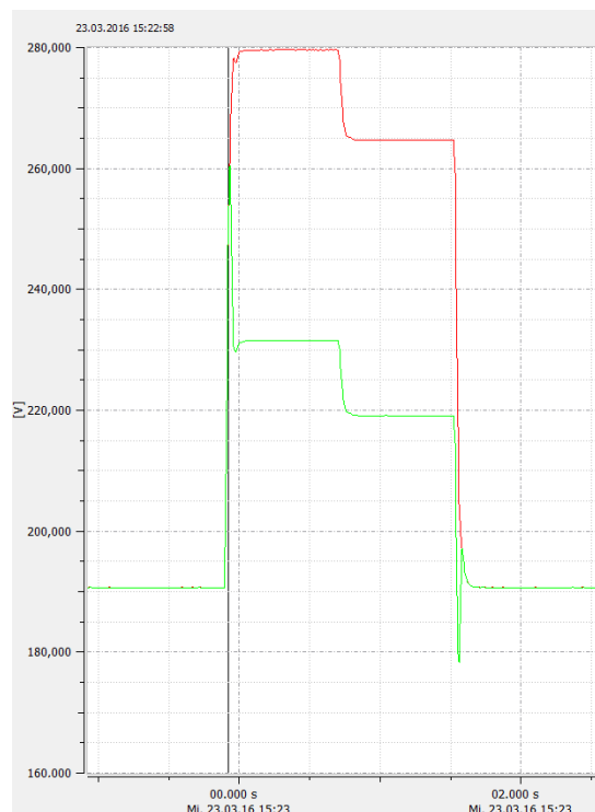
Figure 11. Time reaction of the controller (red: input voltage / green: output voltage)
