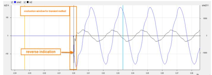
Figure 16 fault record for transient stage, reverse indication; low impedance fault
