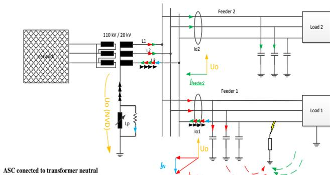
Figure 11  $3I_o$  measured in faulty feeder and healthy feeder vs.  $U_o$
