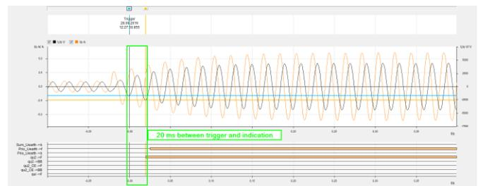
Figure 22 Response time 20 ms after  $U_0$  trigger
