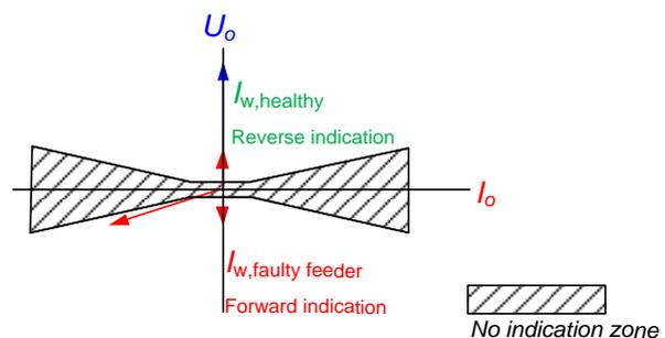
Figure 14 Indication zone for the wattmetric method
