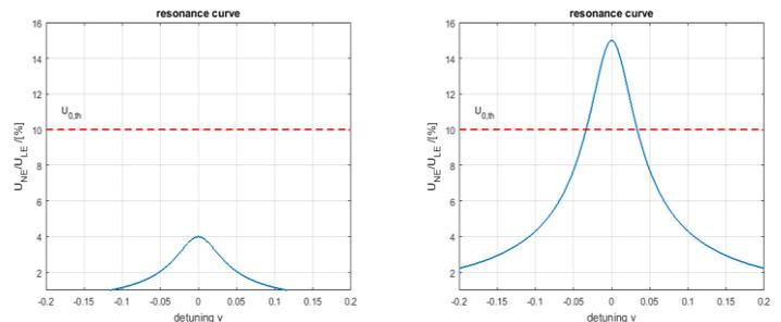
Balanced system  $k = 0,12\%$  (capacitive unbalance) Higher natural unbalance  $k = 0,45\%$  (capacitive unbalance)
