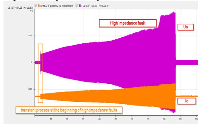
Figure 20 High impedance fault development for 200 s
