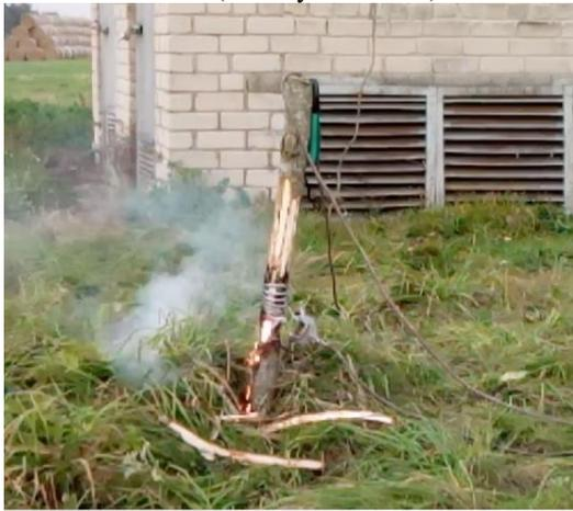
Figure 19 Test site for high impedance fault
