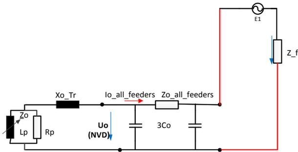
Figure 3 Simplified zero sequence equivalent diagram
