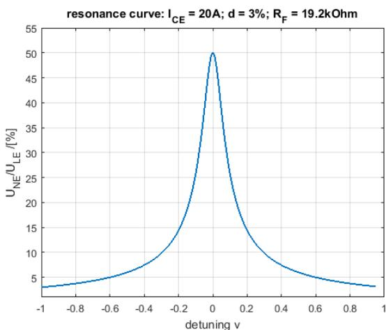
Figure 9 U<sub>o</sub> value for a 19.2 kOhm fault impedance vs. detuning of the ASC; network size is 100 A
