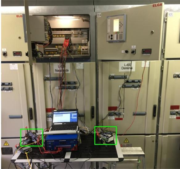
Figure 18 Test setup with EOR-3D for two feeders
