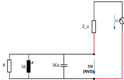
Figure 4 Equivalent zero sequence diagram for sensitivity estimation
