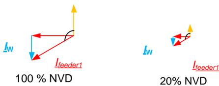
Figure 12 Vector diagram  $U_o$  and  $I_o$ ; low impedance fault vs. high impedance fault
