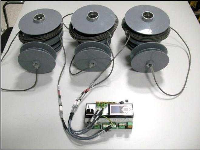
Figure 23 Overhead line combined sensor for phase voltage and current measurement connected to the EOR-3D (A. Eberle)
