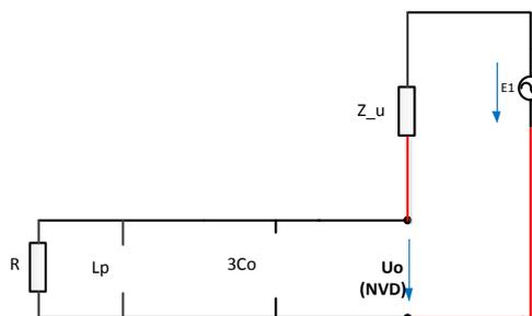
Figure 6 Equivalent diagram at the point of resonance
