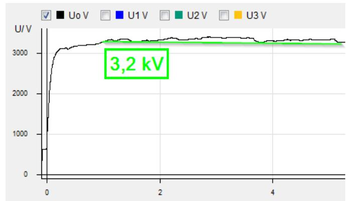
Figure 26 Detuning 0%, 5 kOhm fault impedance
