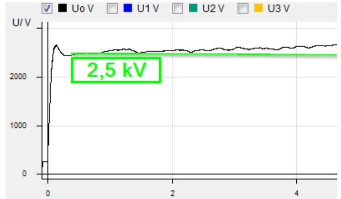
Figure 25 Detuning -10%, 5 kOhm fault impedance
