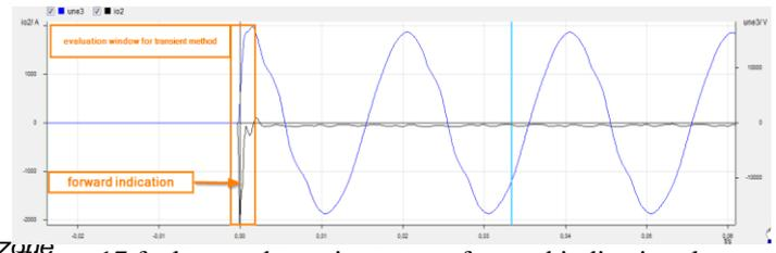
Figure 17 fault record transient stage; forward indication; low impedance fault
