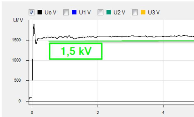
Figure 24 Detuning +40%, 5 kOhm fault impedance
