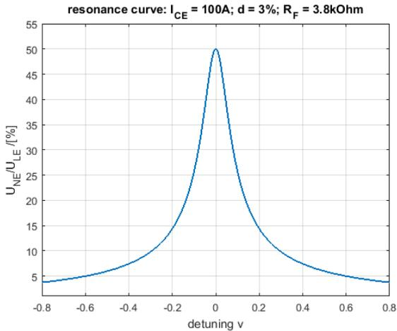
Figure 8 U<sub>o</sub> value for a 3.8 kOhm fault impedance vs. detuning of the ASC; network size 100 A
