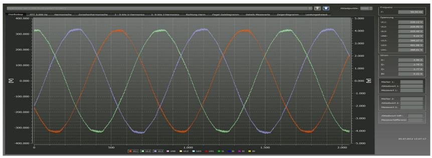
Voltage L1 / L2 / L3 at CPC (Point of Common Coupling) – caused by an Solar Inverter
