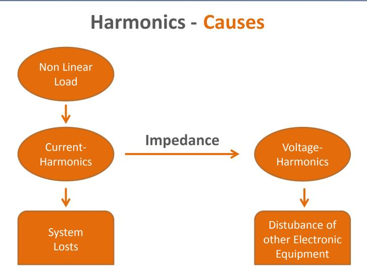
Impedance and Current can be influenced  $\rightarrow$  Voltage is the result! High Impedance **and** non linear Load  $\rightarrow$  High Voltage Harmonic!
