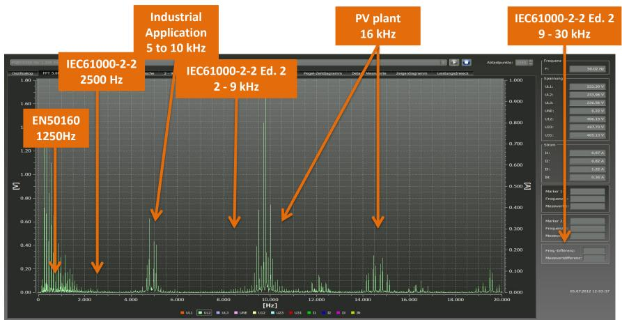
For harmonic disturbances in the range of 30 kHz to 150 kHz there are no compatibility levels defined yet. There have been limit values up to a frequency of 30 kHz for voltage and current harmonics.
