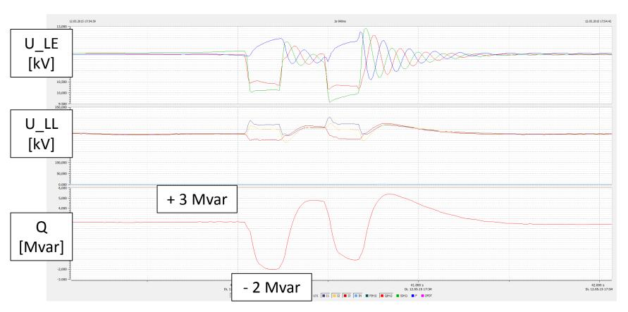
Grid fault measured at a 8 MW wind power plant with PQ Box 200 (1/2 cycle data)
